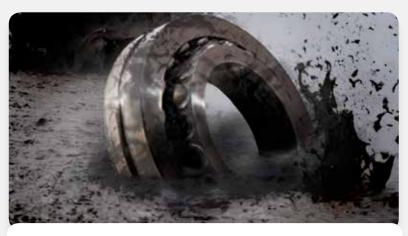
"In our initial testing, we threw sand and gravel into the PCD bearing to see how it would perform. It seemed to like it—just ground up the particles with no problem. In some ways, it actually worked better."
